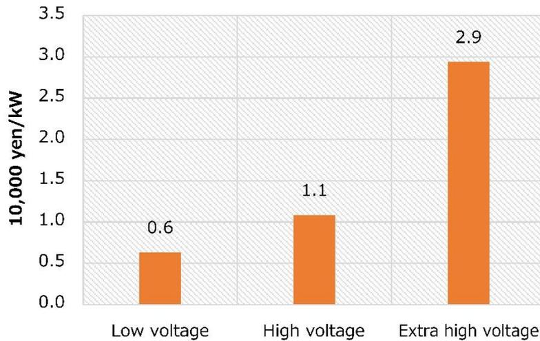
**Fig. 12 Average grid connection cost by voltage class**
