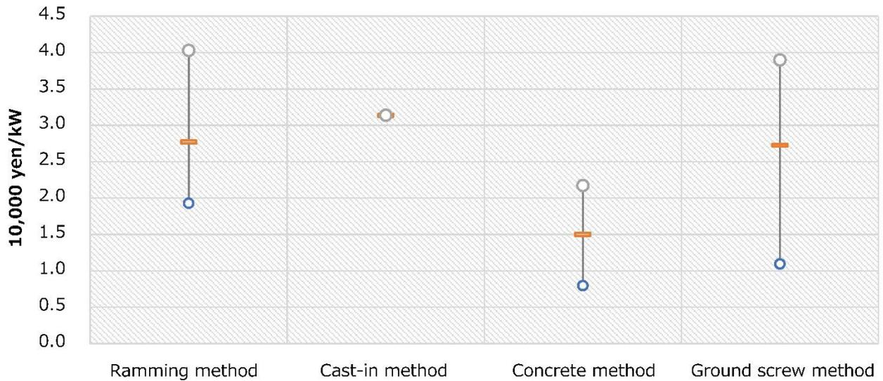
**Fig. 10 Installation unit costs by mounting system type (quartiles)**
