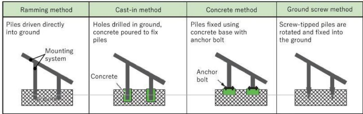
**Fig. 2 Typical mounting system designs and installation methods**
