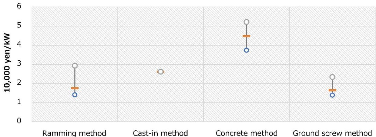
**Fig. 9 Mounting system unit costs by type (quartiles)**
