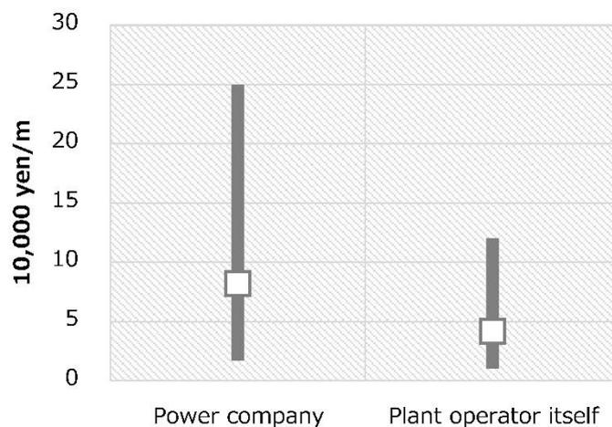
**Fig. 15 Comparison of connection unit costs (10,000 yen/m) at medium-size plants**
