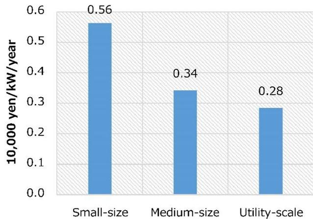
**Figure 20: Average Operation and Maintenance Costs by Plant Size**
