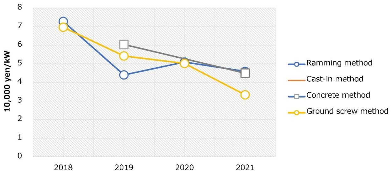
**Fig. 11 Trends in installation-related costs by mounting system type (averages)**
