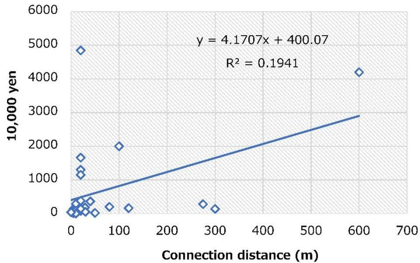
**Fig. 14 Relationship between grid connection costs and connection distance at medium-size plants**
