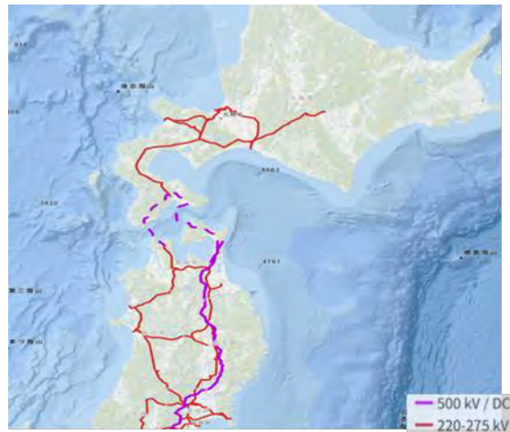
Figure 5. Transmission lines over 220kV in Hokkaido and Tohoku areas
