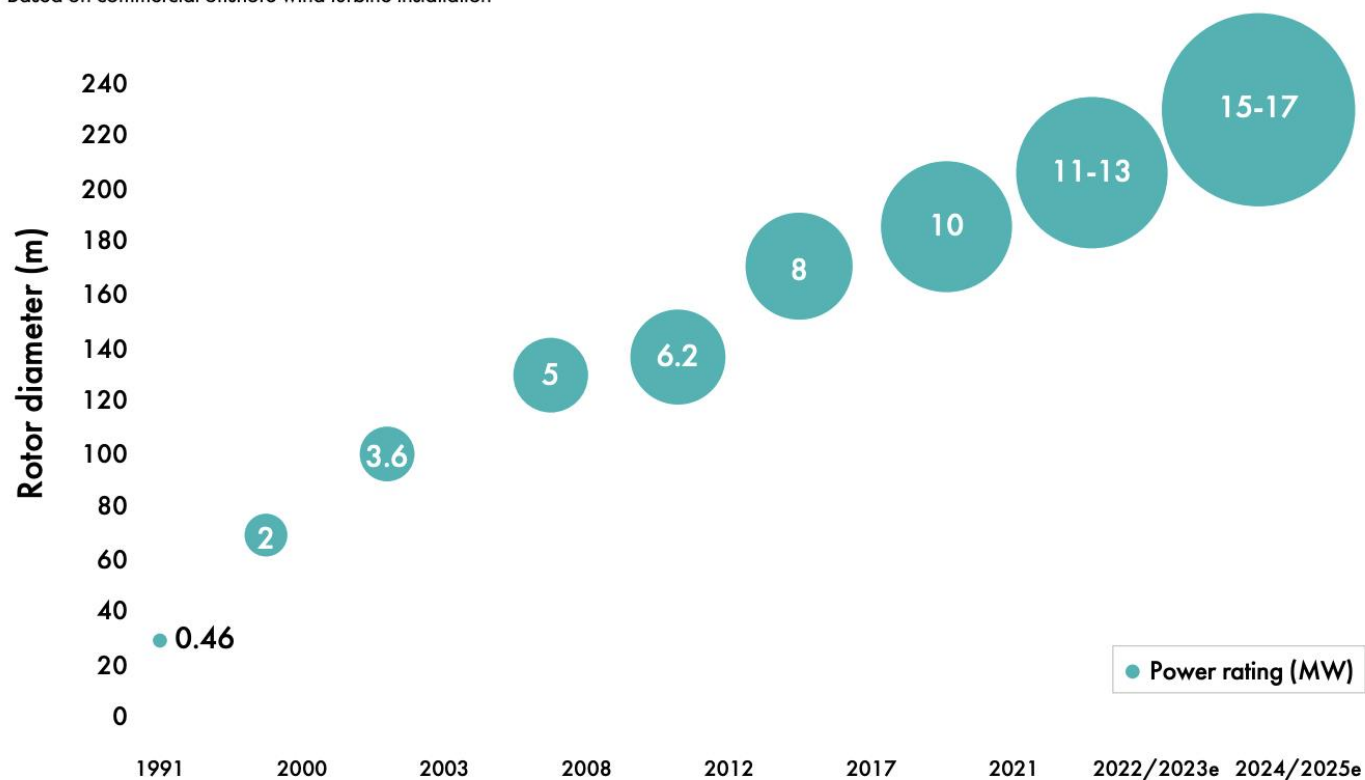
Rotor size and power rating continue to increase Based on commercial offshore wind turbine installation
