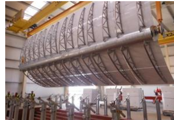
Parabolic Trough Collector Structure assembly line
