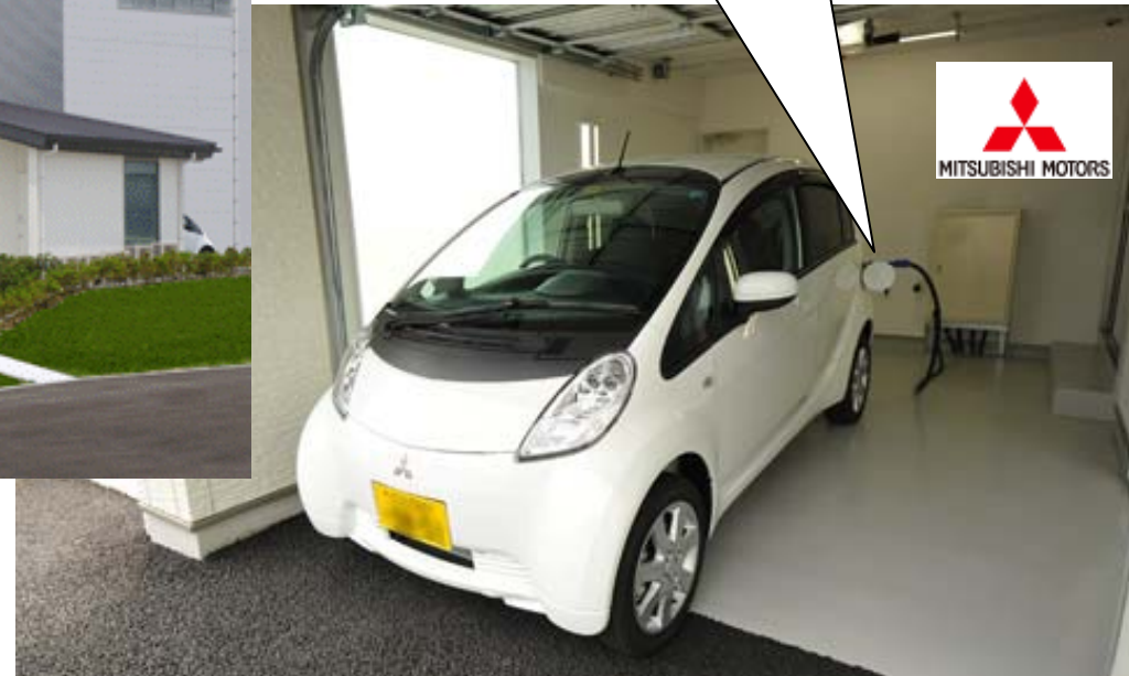
i-MiEV with dischargeable function
