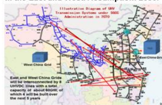
UHV power grid development plan by SGCC: 2 asynchronous power systems will be developed in the East and West. Assumption: 2030.
