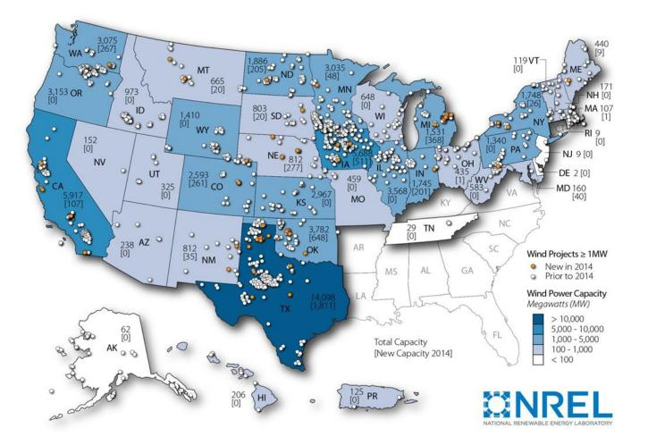
Note: Numbers within states represent cumulative installed wind capacity and, in brackets, annual additions in 2014
